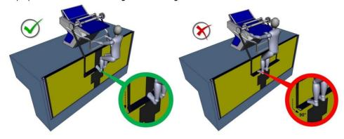
Never put pressure on the Backstroke Ledge when it is in a 90° position.
